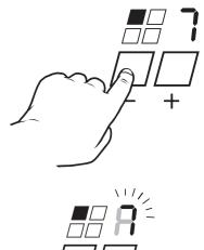
During automatic operation a "A" lights up in the display alternately with the selected cooking setting.
